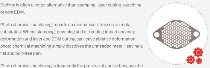
tooling is inexpensive and can be produced very quickly, the parts are very precise and consistent, and the process is particularly effective when the shape of the part is complex and/or the part contains many holes or internal cutouts.
